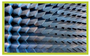
One of the most effective types of radiation absorbent material comprises arrays of pyramid shaped pieces, typically used to house the equipment for performing measurements of EMC.
