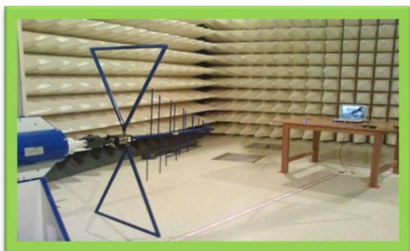
EMC Measurement in Anechoic Chamber
