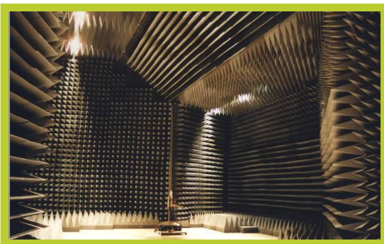
Hands-on session: EMC Measurement in Anechoic Chamber
